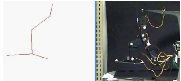
Figure 1. (Right) Cerberus humanoid lower body with position markers. (left) Graphical representation of links throughout the gait using APPAS program
