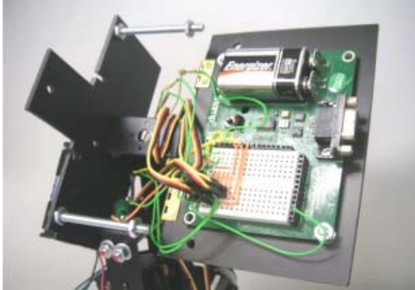
Figure 11. Control board mounted on Cerberus
