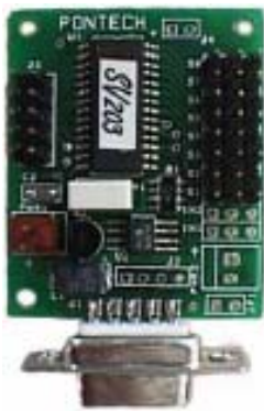
Figure 5: The SV203 Board is very compact, and comes with 8 R/C servo ports and 5 A/D input ports
