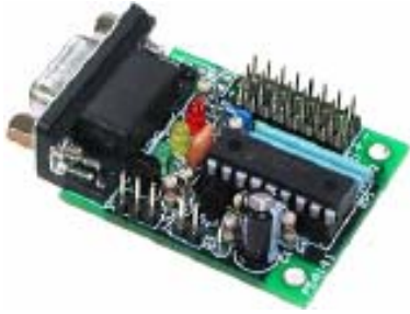
Figure 4: One version of the Pololu Servo Controller can control up to 16 R/C servos
