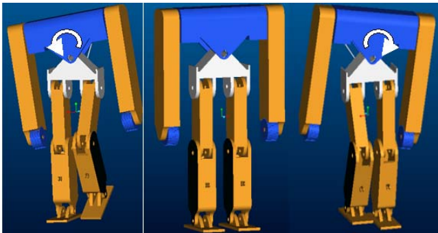
Figure 20. Waist motion for stability in biped walking
