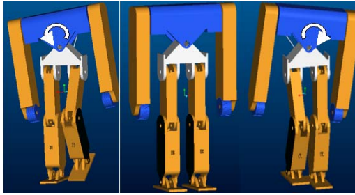
Figure 7. Waist motion for stability in biped walking
