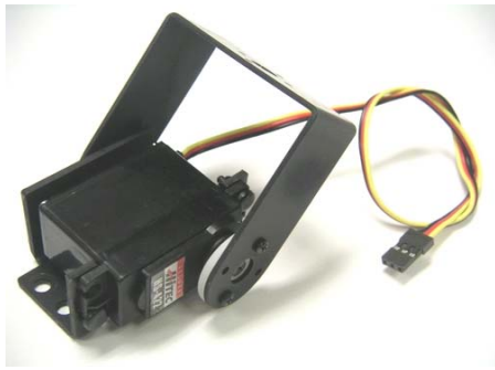
Figure 12. A single limb segment consisting of one standard servo, one servo holder, and one C-shaped bracket
